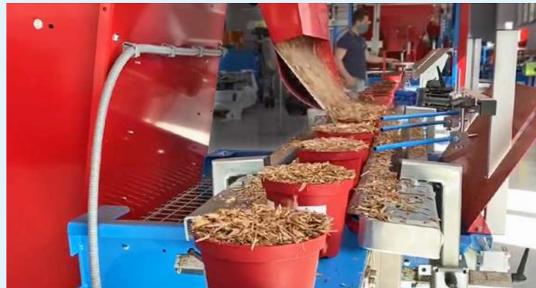
TP2800 in line with IA3500 potting machine configured with central output belt; covering of pots with miscanthus.
