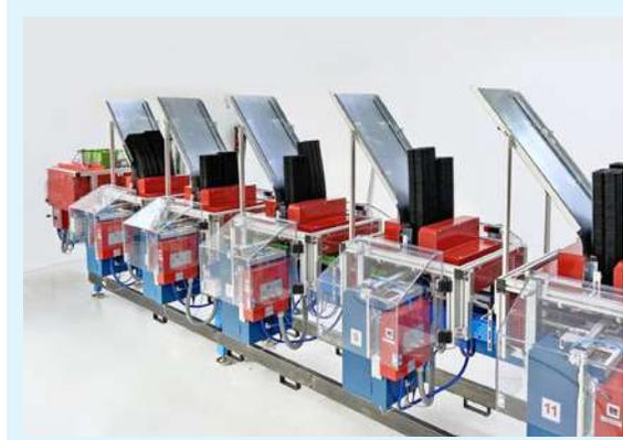
EAC automatic labelling machines serially installed with automatic destackers: the labels are applied to the individual trays before they fall into the tray-holder.
