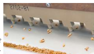
Labyrinth bars, to facilitate the seed positioning.
