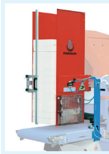
Electropneumatic **destaker with 2-movements**, adjustable with a single crank; for polystyrene trays and trays holder. 48
