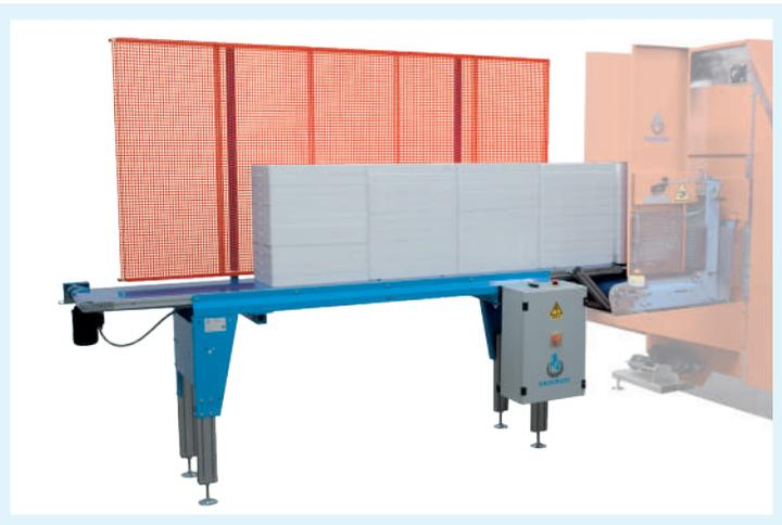
**Feed belt** for single trays or empty stacks for destacker
