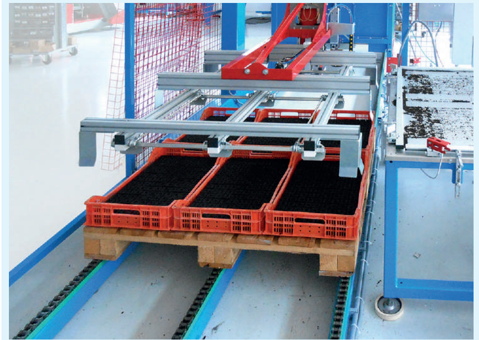
Crates palletizer: pick-up gripper on unloading phase.
