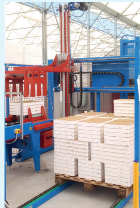
Unloading phase: trays stacked on pallet.
