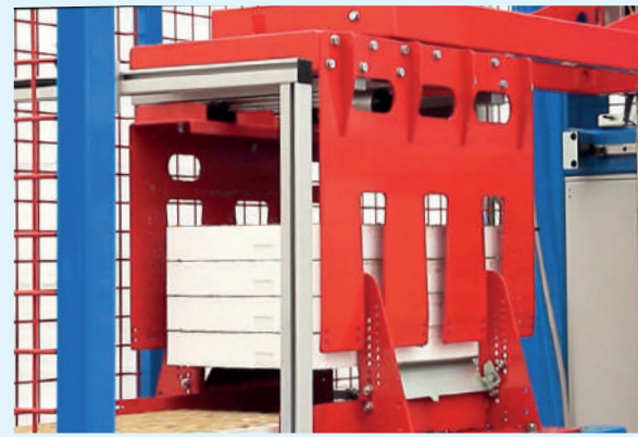
Trays palletizer: pick-up gripper on loading phase.
