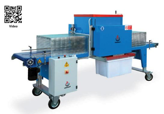
Cutting system and product aspiration with rotating blade. It ensures a precise cut and an excellent cleaning of the trays without any residual leftover.
