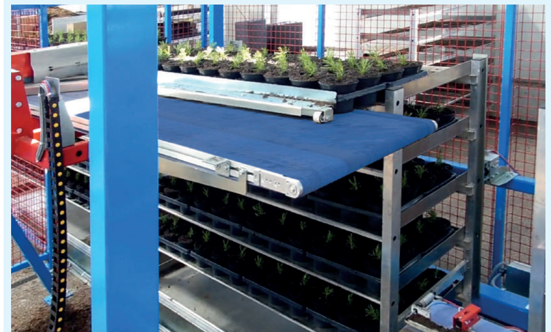
Pots loading phase on trolley shelves.
