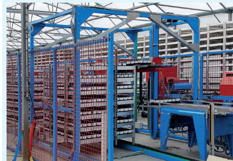
Trolley loader in frame version (rack): advancement system with chain.
