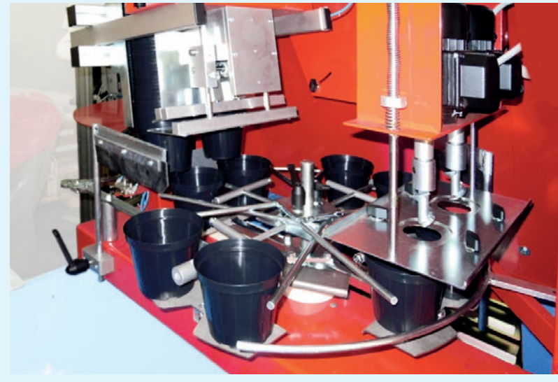
Double head version for pot from diam. 8 to 14 cm: up to 3500 pots/hour.
