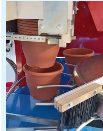
IA3500 single-headed potting machine: it is able to work with pots from 8 to 25 cm , of different shapes and materials.
