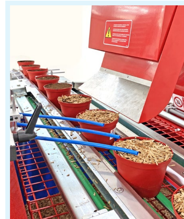
Position and height of leveler tubes are manually adjustable: the excess material removed is automatically put back into circulation .
