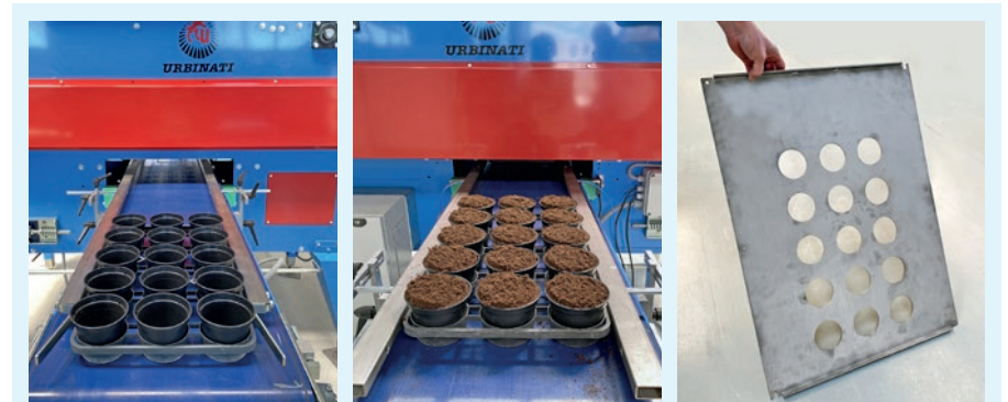
Marketing trays, at filler input and output ; on the right, the relative 15-hole custom filling mask .
