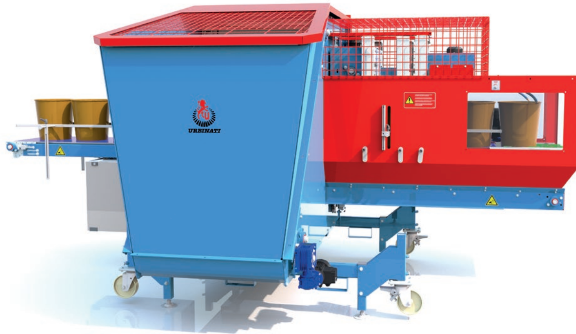
RGV equipped with double air-blower kit for containers cleaning and wheels kit for machine positioning.
