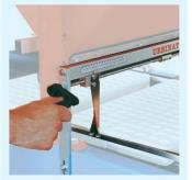
Quick self-centring guide adjustment system, to quickly adapt the guides to the width of the trays in use.
