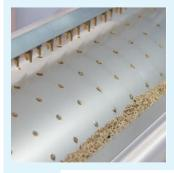
Excellent seeds' singularization thanks to the **double nozzles in** the blowing bar.
