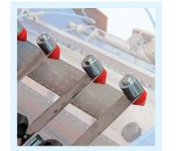
Adjustable speed hammers: the vibration produced optimises the positioning of the seed in the centre of the hole.
