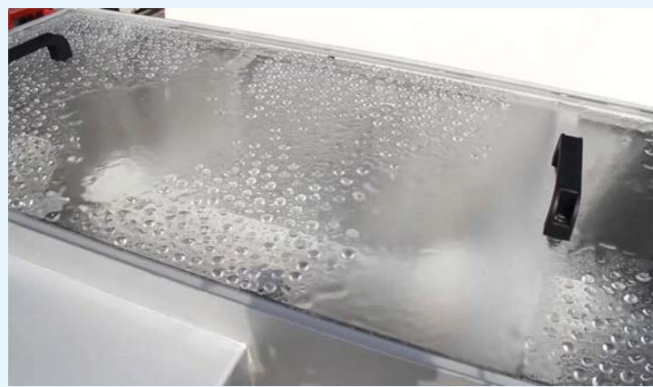
Top plexiglass door for nozzles inspection.
