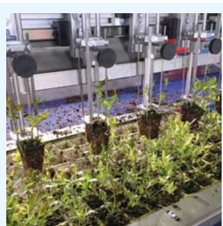
The fingers with the open star are suggested to transplant the forest varieties.
