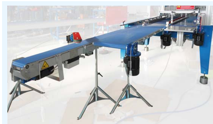
With the 3 axis transplanting selection, the machine can be set with two destination areas: one for trays and the other one for pots.
