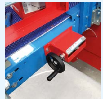
57 Adjustment device for trays with legs.
