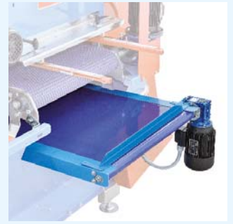
53 Belt for the recycling of the exceeding soil.
