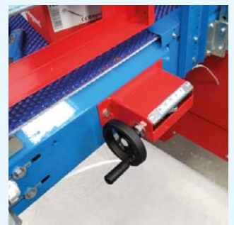
57 Adjustment device for trays with legs.
