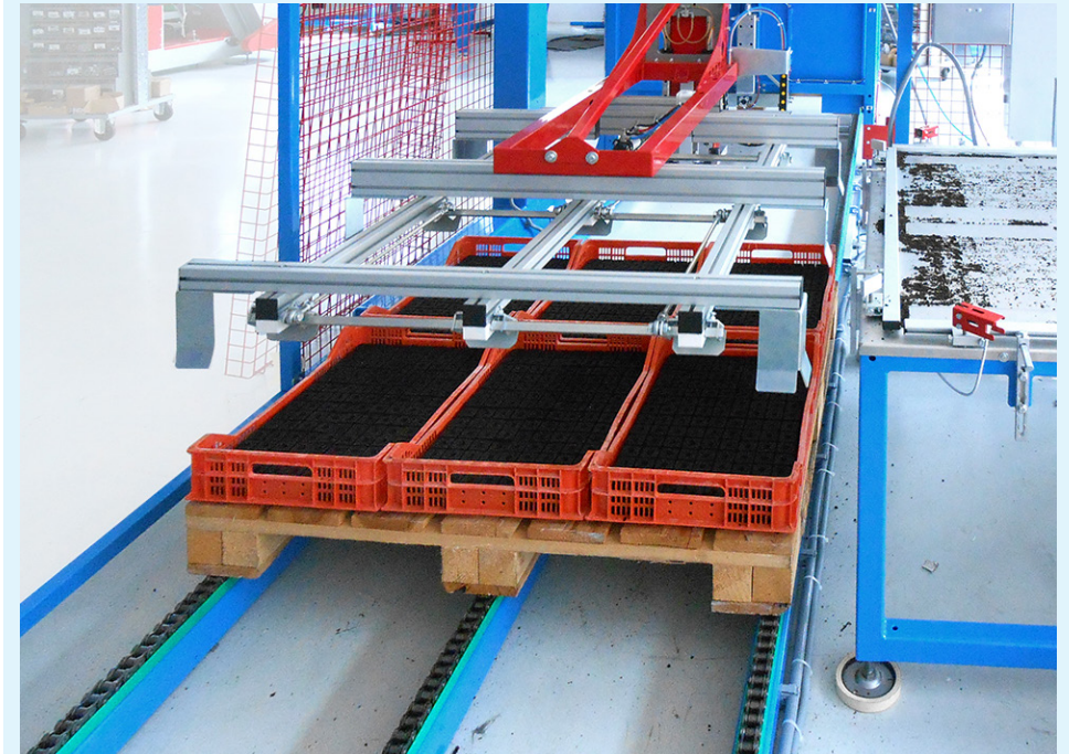
Crates palletizer: pick-up gripper on unloading phase.
