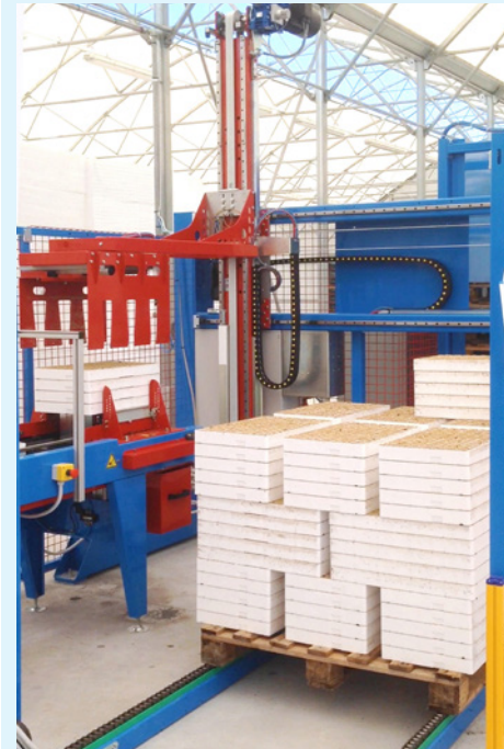
Unloading phase: trays stacked on pallet.
