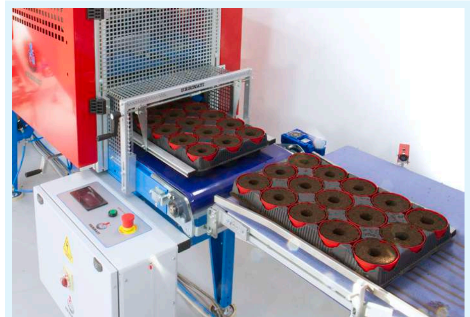
Pots exiting from NIR dibbling machine, inserted in a working line.
