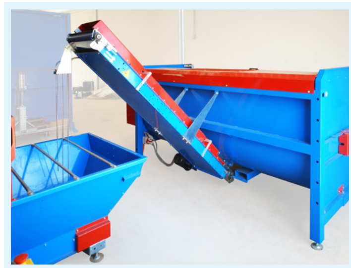
Soil elevator belt with level probes.
