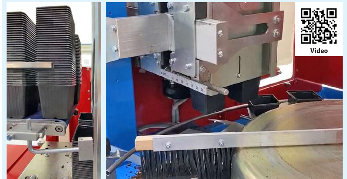
Pots feeding belt, combined with double head for square pots (accessory).
