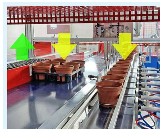
With the third additional conveyor belt for single pots, the machine can be set with two destination area.
