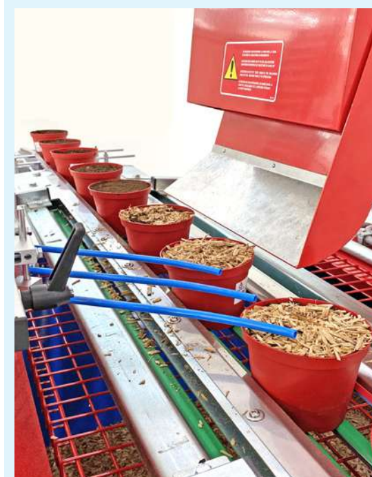
Position and height of leveler tubes are manually adjustable: the excess material removed is automatically put back into circulation.
