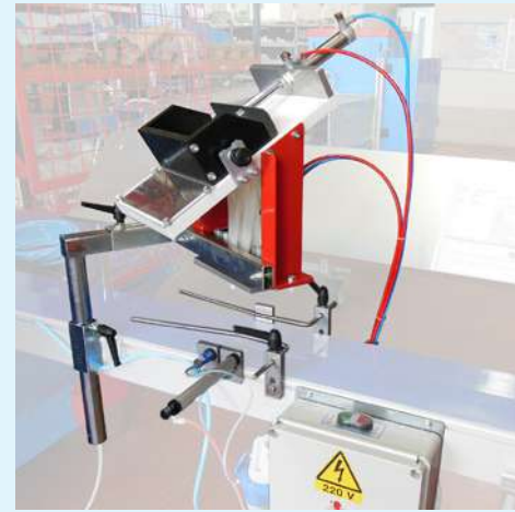
40 Mechanical seeder for aromatic plants, complete with electric panel, pot block and descent seed guided with tubes or spread.
