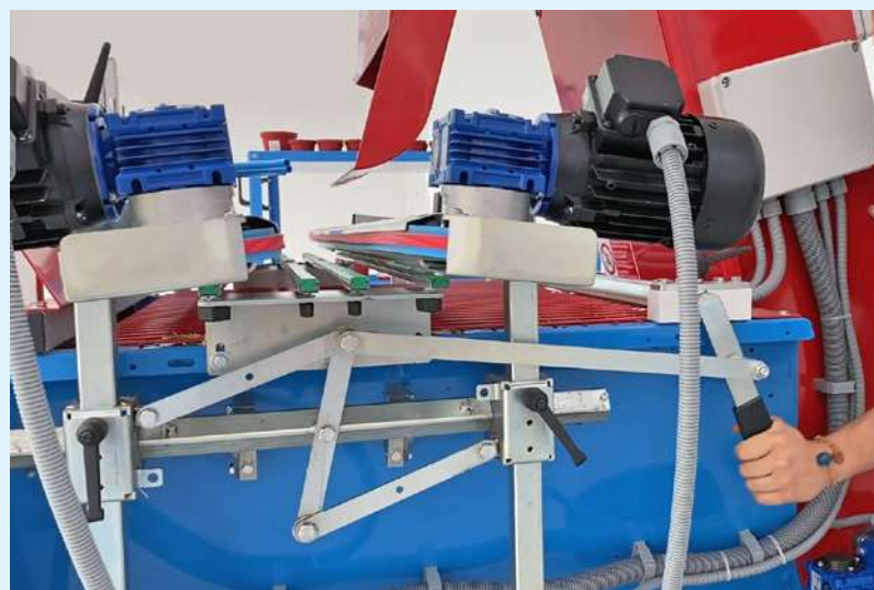
Pot passage width quickly adjustable with a single crank.
